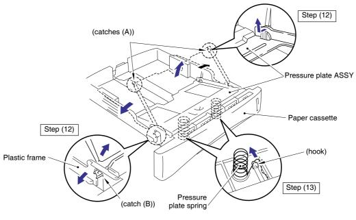
When re-assembling the pressure plate ASSY, ensure that the paper indicator arm is under the pressure plate.
