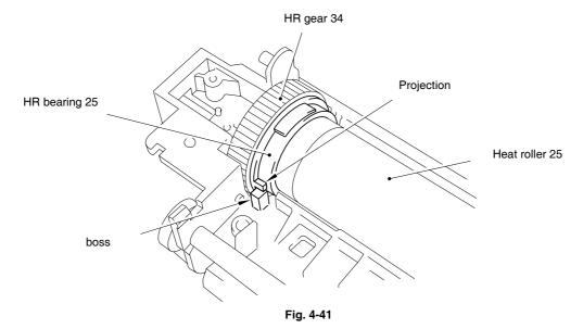
When re-assembling the HR bearing 25 which is assembled at the HR gear 34 side, fix the bearing onto the heat roller 25 so that the embossment whose thickness is 0.5mm is at the
