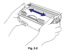
(4) Install the drum unit into the printer and close the front cover.
