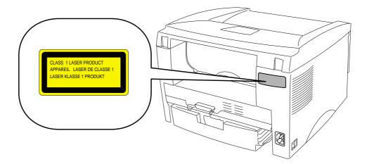
This printer has a laser diode which emits invisible laser radiation in the Laser Unit. The Laser Unit should not be opened without disconnecting the two connectors connected with the AC power supply and laser unit. Since the variable resistor in the laser unit is adjusted in accordance with the standards, never touch it.
