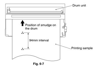
(2) Turn the drum gear by hand while looking at the surface of the photosensitive drum.
